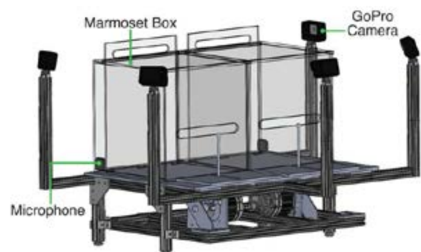
Model of the marmoset pulling apparatus showing its layout, transparent testing boxes, frame structure, video cameras, and microphones. Credit: Olivia Meisner, Nandy lab
