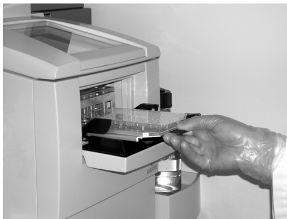
Figure 2-4. Loading the rack tray into the rack tray port.
