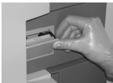
Figure 2-5. Inserting a sensor chip.
