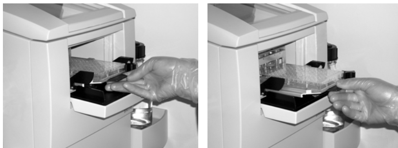
Figure 3-5. Removing the rack tray from the instrument.
