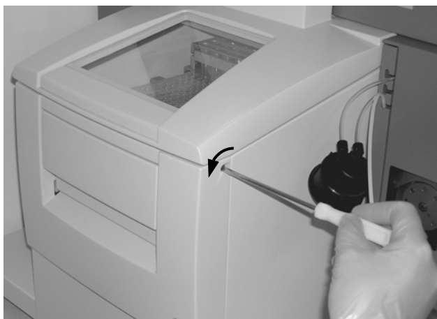
Figure B-8. Opening the sample compartment door.
