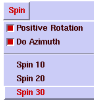
Figure 6.11: The Spin menu automatically computes and inserts camera positions that are 30 degrees apart. This prevents the need to accurately specify each and every position. Spin 10 inserts more camera positions which allows for smoother transitions between camera positions.
