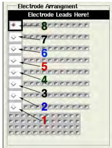
Figure 19.5: Electrode Arrangement Box. Electrodes are numbered from the end farthest away from the leads to the end closest to the leads. Thus, in a strip of electrode, electrode 1 is at the bottom of the Electrode Arrangement display, and the highest numbered electrode is at the top.
