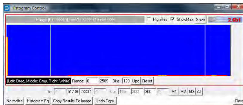
Figure 7.3: The “Show Max” box is checked which shows the tallest bin. In this case, the tallest bin is the background. Figure 7.2 shows a histogram for the same image with the Show Max checkbox unchecked.
