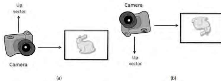
Figure 2.2: The Up-vector for the Camera. The left image shows the result of the camera vector pointing upwards. The right image shows the result of the up-vector pointing downwards. The projected image on the view plane is inverted.
