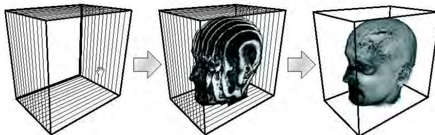
Figure 2.7: This figure shows a schematic of the axis-aligned polygons on the left, that are texture-mapped and blended to get a volume rendered image of the data.
