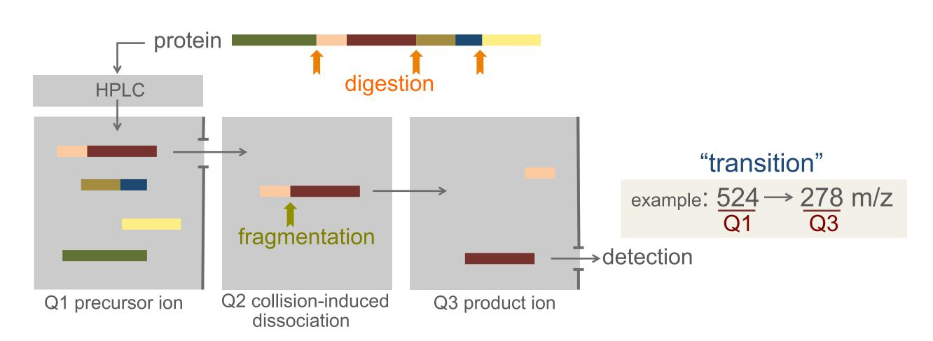
MRM is highly specific assay method for detecting analytes of interest utilizing, most predominantly, a triple quadrupole-based mass spectrometer. Q1 is set to transmit only the parent m/z of the peptide, the fragmentation via collisional induced dissociation occurs in Q2, and Q3 is set to transmit this diagnostic fragment only. The specific combination of m/z associated with the parent and fragment ion selected are referred to as a "transition".
