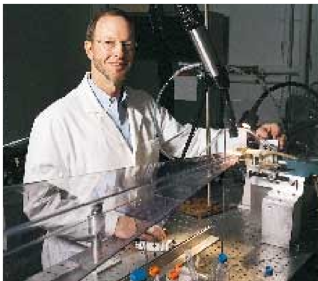
Donald Engelman and a Rochester colleague have shown there's more than one way to fold a protein. Engelman used a small-angle X-ray scattering instrument, pictured here, to measure the size and shape of proteins in solution.
