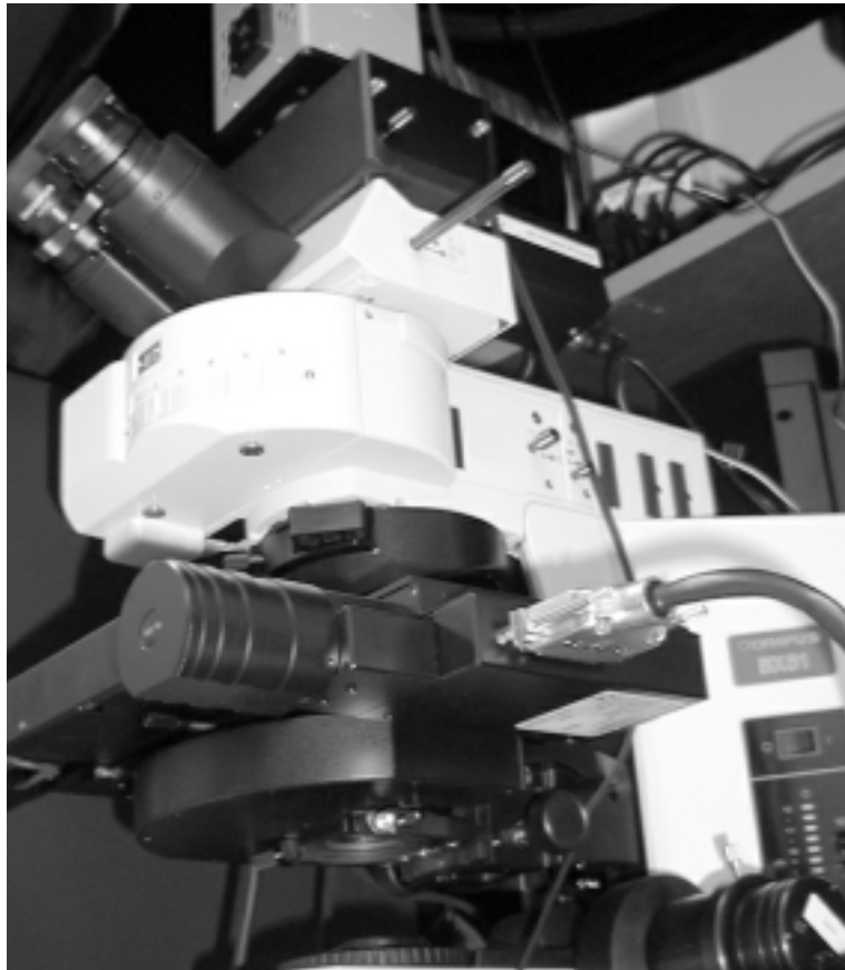
Above The PM1000 is pictured above. It is designed to measure protein concentrations in tissue samples.
