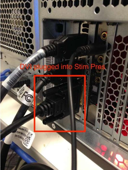
Figure 2. DVI cable plugged into the back of the Stimulus Presentation computer
