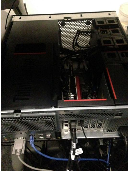
3. Lift up side handles, disconnect hard drive from mounting bracket, and label it (ie. original hard drive)
