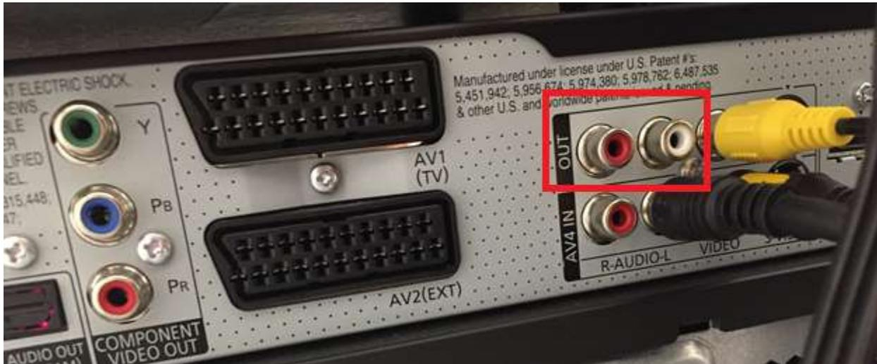
Figure 1. Photo of the back of the DVD player with the RCA output ports boxed in red
