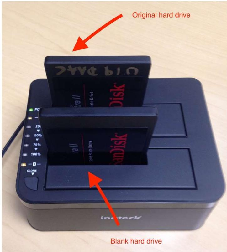
6. Press “clone” button on the product for about 3 seconds, release and the LED indicator of 100% will light up, and quickly click “Clone”
